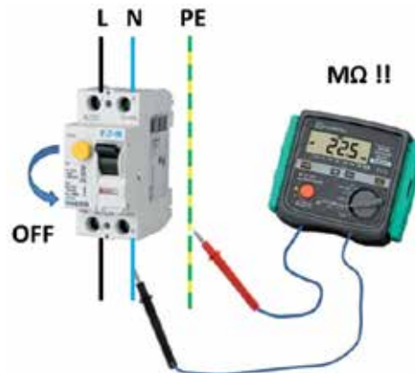
Fig. 92 Check of separation of PE and N conductors after a tripped RCD
