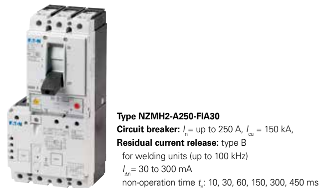
Fig. 41 Circuit breakers with residual current protection for industrial use (CBR)
