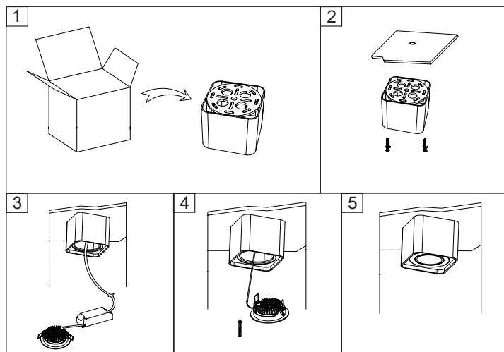
1. When you have removed the surface-mounted luminaire from the packaging, mark on the ceiling where you want to place the luminaire.
