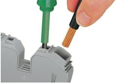
Terminating a 35 mm<sup>2</sup> (2 AWG) conductor.
