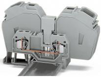
Commoning with step-down jumper (283-414) from 285 Series (35 mm<sup>2</sup>/2 AWG) to 281 Series terminal blocks (4 mm<sup>2</sup>/12 AWG).
