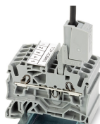
Testing tap (Item No. 2009-182) for tool-free connection of test cables up to 2.5 mm 2 (12 AWG) – compatible with 2000 to 2016 Series
