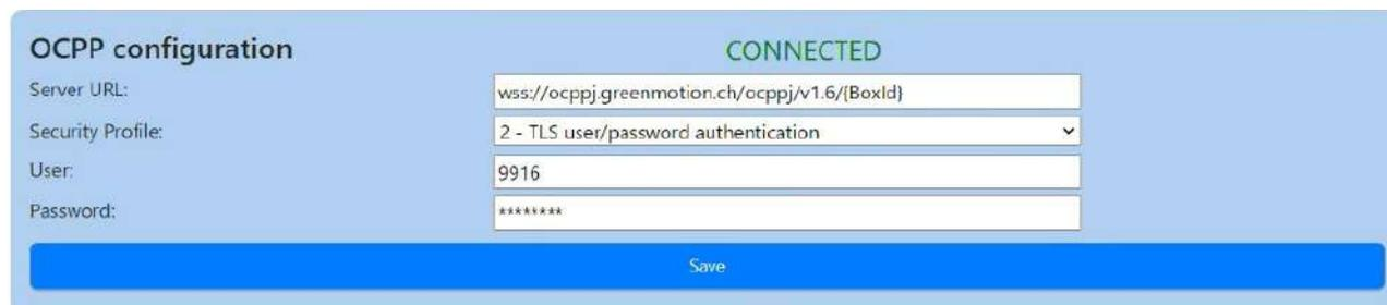
The screenshot shows a configuration window titled "OCPP configuration" with a "CONNECTED" status indicator. It contains four input fields: "Server URL" with the value "wss://ocppj.greenmotion.ch/ocppj/v1.6/{BoxId}", "Security Profile" with a dropdown menu showing "2 - TLS user/password authentication", "User" with the value "9916", and "Password" with masked characters "\*\*\*\*\*". A blue "Save" button is located at the bottom of the form.
