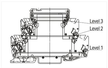
Universal modular component plug housing, as rail-mount terminal block – transparent cover
