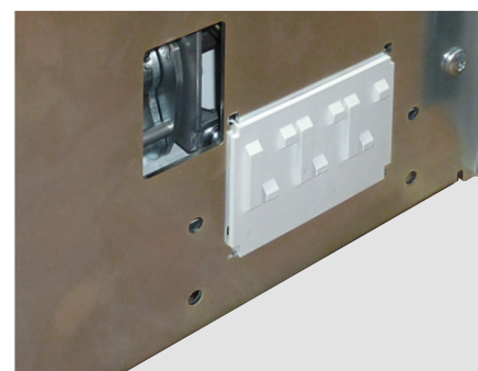
The plate mounted under the DMX 3 actuates the contacts during the inserted and draw-out operations.
