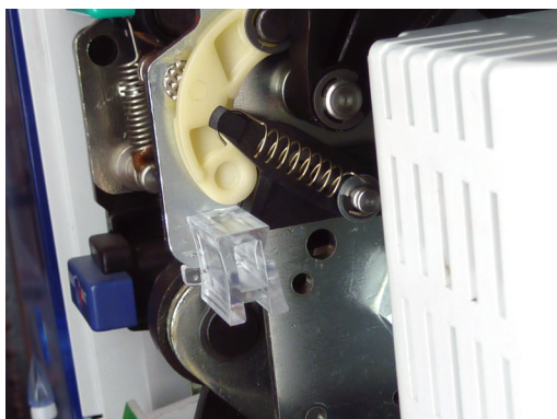
Accessory for correct adjustment of the supply inverter connecting rod.
