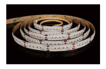
24V, flexible LED strip (14LED/step =38.46mm) with 3M adhesive tape on the back for easy installed.. Very good color reproduction with CRI>95. "One Bin Only" within 3 MacAdam guarantees constant color temperature and high light quality at a lifetime of 54,000 hours (L<sub>70</sub>). Double-layer FPC(2Oz) for good heat dissipation.
