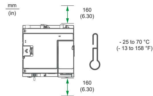
**en** Install the meter in an area where the ambient temperature is maintained according to the temperature specification. Leave space for wiring and access.
