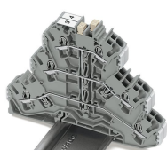
Commoning three levels via triple-deck vertical jumper (2002-493).
