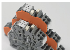
Created for double- and triple-deck TOPJOB® S Terminal Blocks, the vertical jumpers can common two or three levels. Clearly marked numerals ("2" and "3") distinguish the double-deck (2002-0492) and triple-deck vertical jumpers (2002-0493), even when inserted.
