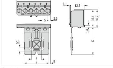
Dimensions in mm L = pole no. x pin spacing
