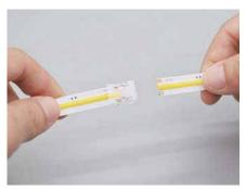
Insert each ends of led strips into the end of the connection terminal respectively, make sure the metal clip is on the same side as the metal solder pad of led strip.
