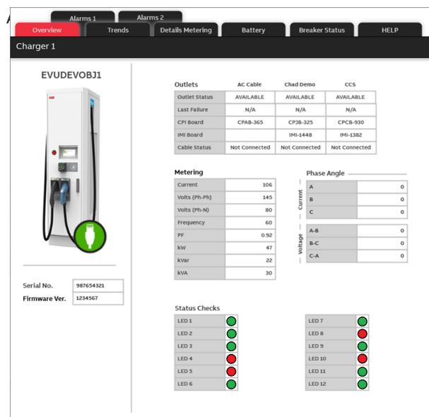
The HMI provides the capability to manage individual parking sites through different interface tabs.
