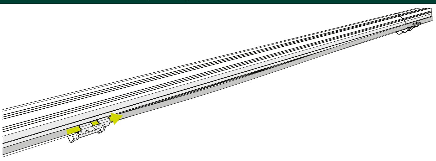
7 Place the panel on the rails and Slide the panel against the clamps.
