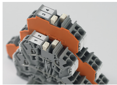
Created for double- and triple-deck TOP-JOB® S Terminal Blocks, the vertical jumpers can common two or three levels. Clearly marked numerals (“2” and “3”) distinguish the double-deck (Item No. 2002-0492) and triple-deck vertical jumpers (Item No. 2002-0493), even when inserted.
