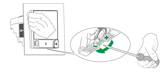
2. Carefully pull the display away, far enough to access the cable connector on the display.
