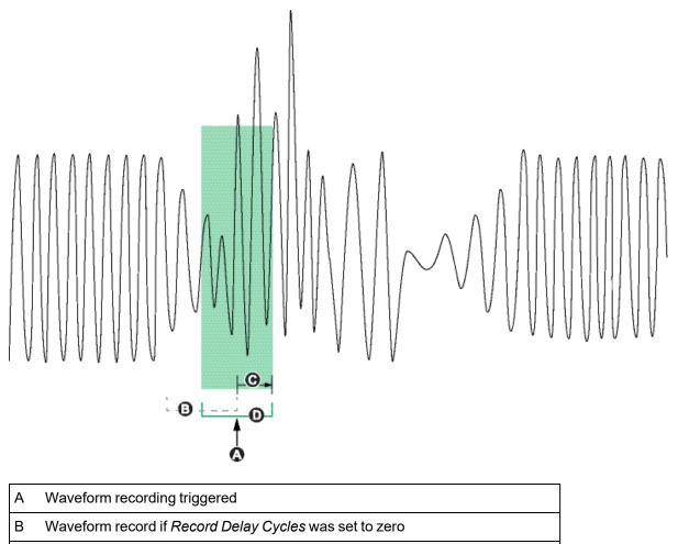
C Delay period (number of cycles specified in Record Delay Cycles setup register)
