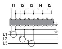
For a 3-phase 3-wire system, the meter measures the residual current for Ground at I4.
