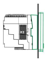
1. Holding the display, turn the tightening wheel with a flat-head screwdriver until it disengages from the display.
