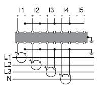
For a 3-phase 4-wire system, the meter measures the residual current for Ground at I5.
