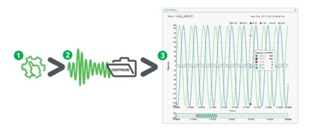
1. Enable waveform 2. A waveform is captured when 3. View the waveform on the capture on your meter a power quality event occurs
