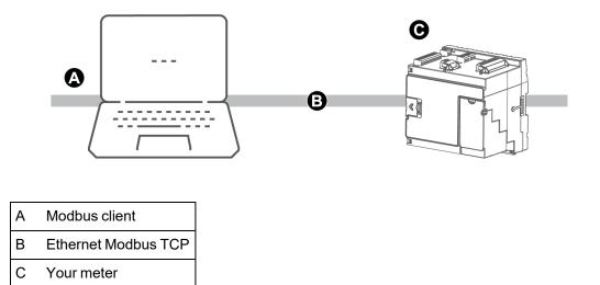
Your meter does not require any Modbus-specific configuration to act as a Modbus server device over Ethernet.
