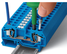
CAGE CLAMP® connection Inserting a conductor. With ferruled conductors, it is necessary to use a terminal block one size larger than the conductor's nominal cross-section.
