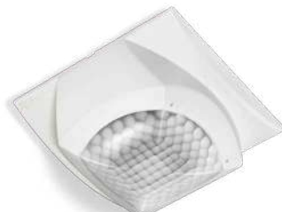
Type 18.51 • PIR movement and presence detectors • Push-in terminals • Standard version or with DALI or KNX interface • External switching push-button connection • Programmable and adjustable via the FINDER TOOLBOX app (iOS and Android) • Programmable via Bluetooth LE (Low Energy)
