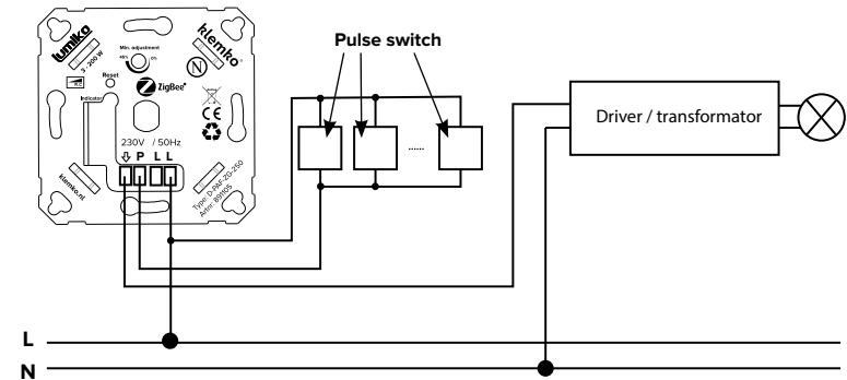
Several pulse-based switches can be connected between the phase L and the connection P. This allows the lighting to be switched on/off or dimmed at several points.
