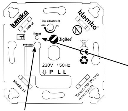
Reset switch for connecting to the network and disconnecting to factory settings.
