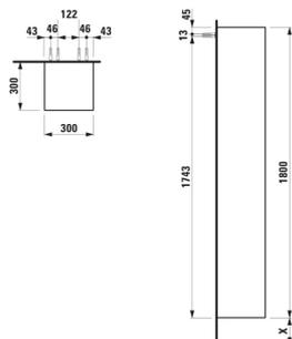
X = The exact height must be set during installation.
