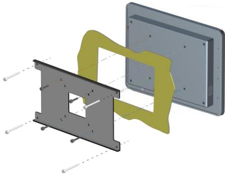
Place the back plate against the back of the eXplore unit and re-insert the 4 x VESA screws.
