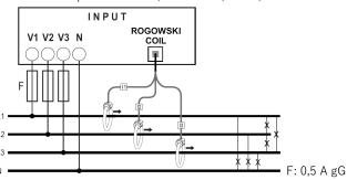
. Rogowski coils cables length (see § Overall Dimensions) in addition to the extension cables, allow you to put EMS CX<sup>3</sup> Measure modules everywhere in the installation.
