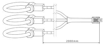
This length can be stretched via the Extension cable + connector up to 5 meters (2 m of Rogowski cable and un to 3 m of extension)
