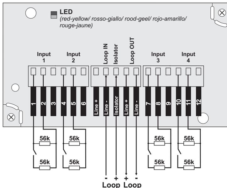
ATTENTION: When you use the integrated short circuit isolation module connect one of the "+Loop" loop lead to the "Isolator" terminal of the module!
