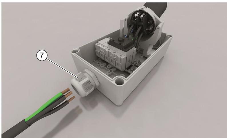
7. The terminals are open at the time of delivery. Guide the bare individual conductors into the opening and tighten the screws with the minimum torque (16A and 32A design: at least 0.8 Nm; 63A design: at least 2.0 Nm; 125A design: at least 4.0 Nm). Take care to see that only the bare individual conductor (without insulation) is clamped. Pay attention to the marking of the terminals and ensure that the assignment of the individual conductors to the terminals is correct.
