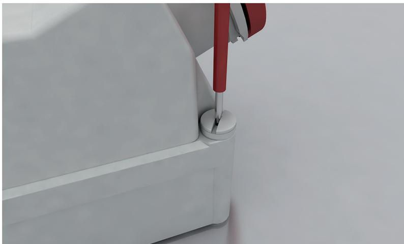
3. Loosen the screws and pull out the individual conductors from the terminals.
