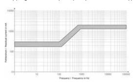
Tripping current frequency response 500 mA Type S/Bfq
