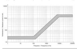
Tripping current frequency response 100 mA Type B
