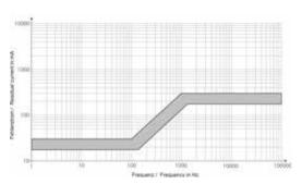
Tripping current frequency response 30 mA Type G/B+
