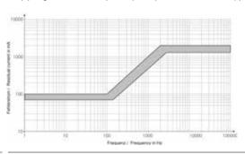
Tripping current frequency response 300 mA Type S/Bfq
