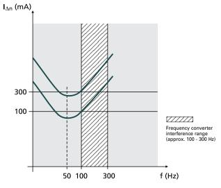
This sample tripping characteristic of a 100 mA RCD and a 300 mA RCD shows the following: In the frequency range around 50 Hz, the RCDs trip as required (50 - 100 % of the indicated  $I_{\Delta n}$ ).
