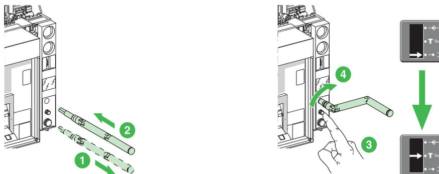
1. The device is in disconnected position. Remove the racking handle from its storage space.
