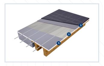
If you opt for a **cast floor**, a self-levelling top coat is applied first or a gypsum fiberboard is used. Follow the instructions for the leveler as described above. The gypsum fiberboard is glued to the Secor panels. For this, use a primer first for adhesion of the glue. The gypsum fiber boards have a minimum thickness of 10 mm. The self-levelling floor is placed on top of these gypsum fiber boards.
