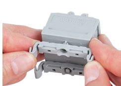
Snapping a mounting foot (209-120) to a terminal strip with snap-in mounting feet. (Distance between mounting feet: approx. 20 ... 25 mm)
