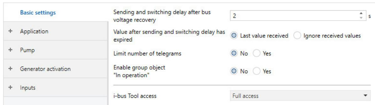
Fig. 5: Parameter window Basic settings
