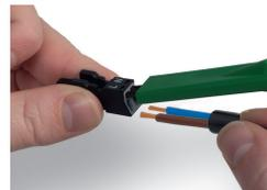
To terminate fine-stranded conductors, open clamping units via operating tool (890-382) and insert stripped conductors until they hit backstop. Terminate solid conductors by simply pushing them in.
