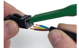
To terminate fine-stranded conductors, open clamping units via operating tool (890-383) and insert stripped conductors until they hit backstop. Terminate solid conductors by simply pushing them in.
