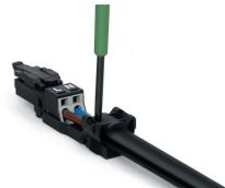
Push down strain relief clamp with 2.5 mm screwdriver alternately on both sides.
