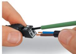
To terminate fine-stranded conductors, open the clamping unit via screwdriver – 2.5 mm blade width – and insert a stripped conductor until it hits the backstop. Terminate solid conductors by simply pushing them in.
