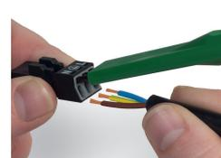
1. Strip length, outer insulation = 30 mm (2-pole), 37 mm (3-pole), 45 mm (4- and 5-pole)
