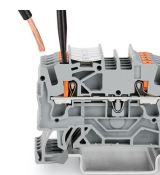
Insert fine-stranded conductors via operating tool.
