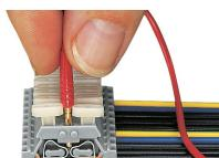
Testing with voltage tester.
