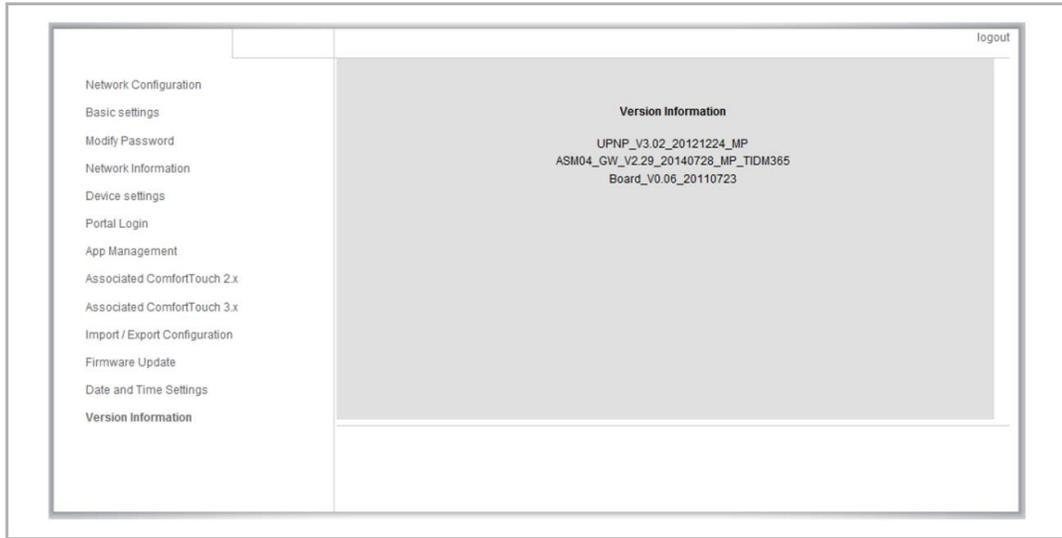
The "Version Information" configuration page provides information about the hardware and software components of the IP gateway and is required for service purposes or error diagnostics.
