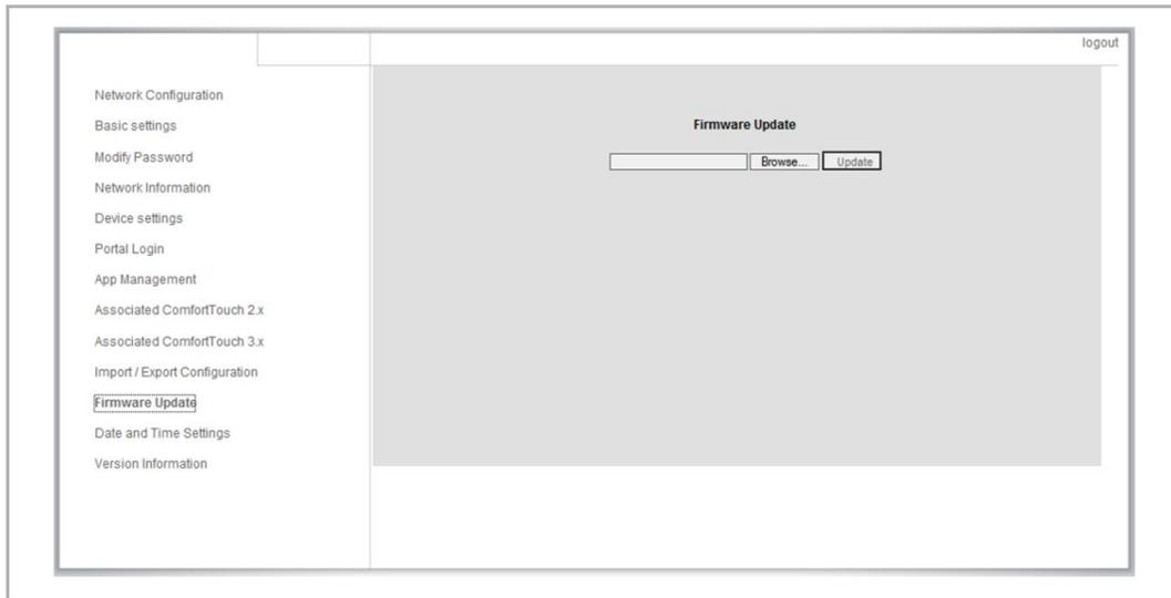
The IP gateway has the option to manually update the device software.
