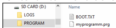
Fig. 73: microSD memory card drive with PROGRAM folder contains BOOT.TXT and compiled test.prg program
