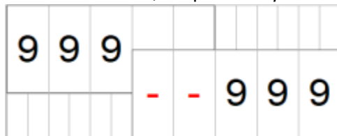
Fig. 230: Two value displays with two characters overlapping
