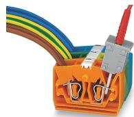
Testing by touch contact to the CAGE CLAMP® spring (limited to 0.5 A and 48 V test voltage) – test pins are not protected against accidental contact.
