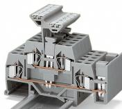
A vertical jumper commons the upper and lower decks, creating a 4-conductor commoned through terminal block in one housing. Two adjacent terminals may be commoned together on the same deck using a push-in adjacent jumper.
