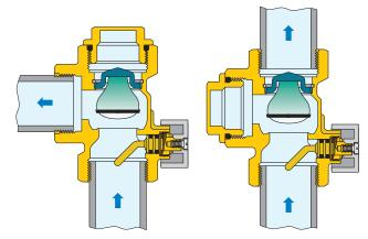
The valve should be installed in accordance with the flow direction indicated by the arrow on the valve body. The valve can be used with straight or angled connections, by moving the third way sealing cap. The valve should be installed with the check valve axis vertically, in accordance with one of the two diagrams provided.
