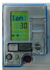
Current setting and earth leakage module threshold.
