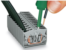
CAGE CLAMP® connection Inserting a conductor. With ferruled conductors, it is necessary to use a terminal block one size smaller than the conductor's nominal cross-section.
