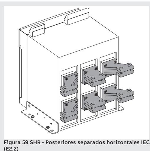
Figura 59 SHR - Posteriores separados horizontales IEC (E2.2)
