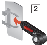
Figure 8.18 Handle and spare fuses can be stored on the motorized switch-fuse by mounting the accessory OTVS_
