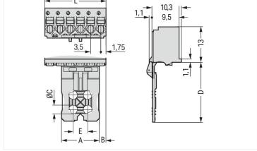
Dimensions in mm L = (pole no. – 1) x pin spacing
