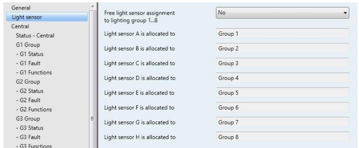
If several light sensors are assigned to an output, it is necessary to define which sensor value is used as the actual value (input variable) for the control circuit.
