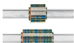
With a terminal block width of just 5 mm, an effective width of just 2.5 mm for terminal blocks of same or different potentials can be realized for conductors ranging 0.08 mm<sup>2</sup> ... 2.5 mm<sup>2</sup> (28 ... 14 AWG).
