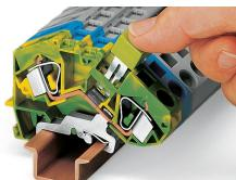
Commoning ground conductor terminal blocks with through terminal blocks is possible in one direction only (via rear side of terminal block) using adjacent jumpers. WAGO recommends using yellow-green adjacent jumpers in addition to the required marking of these blocks.
