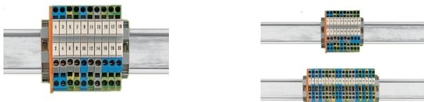
With a terminal block width of just 5 mm, an effective width of just 2.5 mm for terminal blocks of same or different potentials can be realized for conductors ranging 0.08 mm<sup>2</sup> ... 2.5 mm<sup>2</sup> (28 ... 14 AWG).
