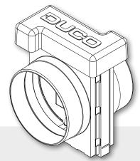
The Humidity Box Sensor can be incorporated in the DucoBox Energy Comfort 325 extract duct (ETA). The box sensor housing has two 160 mm diameter connections (M). The box sensor is to be connected to the DucoBox Energy Comfort 325 control card via the power supply and communication cable supplied.
