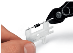
Cutting component to the proper length.
