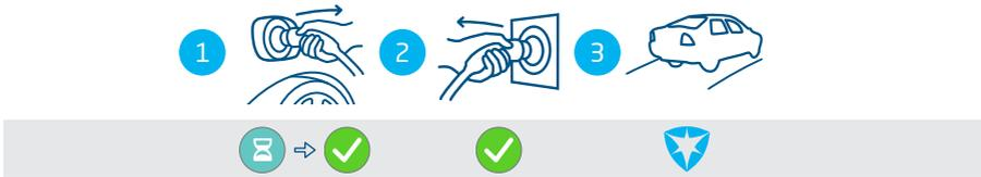
Figure 4.2: Stopping the charging process without RFID card. Symbols shown on user interface
