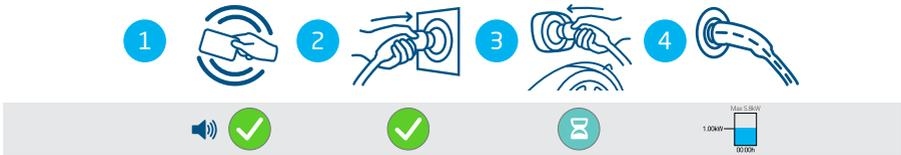
Figure 4.3: Starting the charging process with user authorization / RFID card. Symbols shown on the user interface
