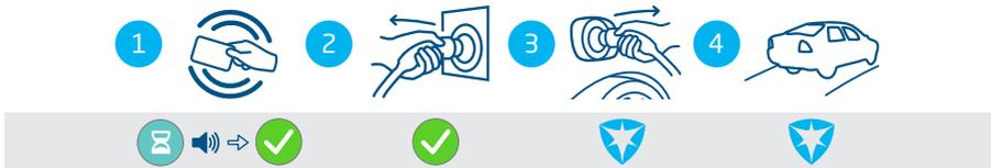
Figure 4.4: Stopping the charging process with user authorization / RFID card. Symbols shown on the user interface
